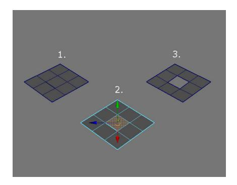
3. Navigate to Edit Mesh – Append to Polygon Tool. Select an edge that borders the opening; purple triangles will appear, indicating where you can append a face or polygon to. Select the triangle directly across from your initial selection; a pink fill will appear inside the opening. Press Enter to confirm.
