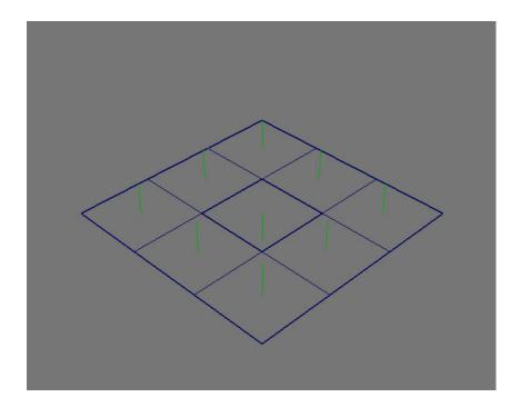
As can be seen in my example above, with the normals display turned on, the center polygon has an inverted normal with a resultant 4 border edges.
