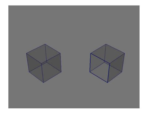
The cube on the left has no border edges because each of its edges form an enclosure of polygons; what's called a "closed mesh". When a polygon is removed, as seen on the right, however, a loop of four border edges is produced because an opening into space is made; what's called an "open mesh".
