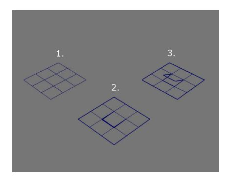
At first glance, the plane on the left appears normal with all of its edges sharing one vertex. With border edges turned on however, we can see that three edges are in fact not, and that the middle polygon is thus not connected to the ones surrounding it.
